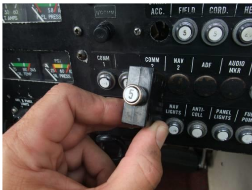
5 Amp Circuit breaker
